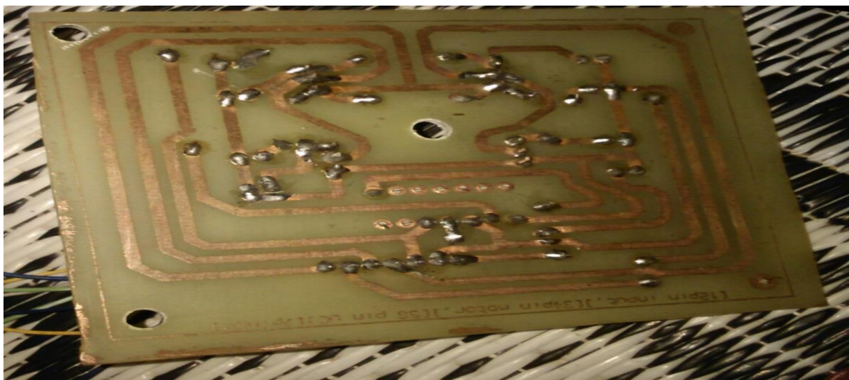
Figure 9. Fabricated H-bridge PCB used for motor control.
