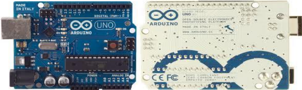
Figure 11. Arduino UNO board used in the implementation. Features used are
